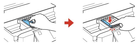
9. Once you replace all the cartridges that need replacing, close the scanner unit.
